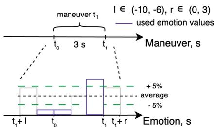
Fig. 5. The scheme of the algorithm for estimating the emotional expression without taking into account the individual characteristics of the driver
