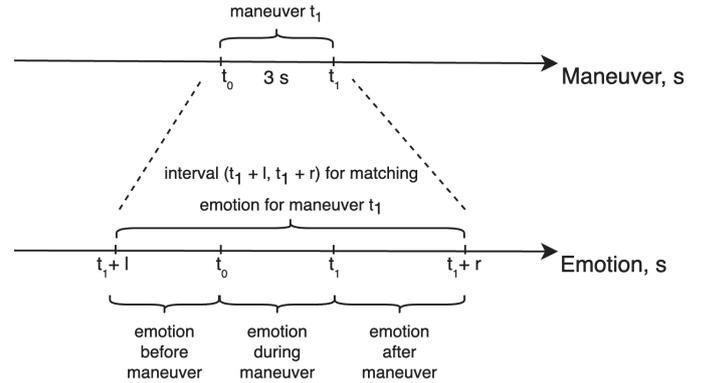
Fig. 2. The model of matching vehicle maneuvers with the driver's emotions at that moment
