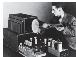
Fig. 11. Ardenne with a Braun tube in his laboratory, 1931. The earliest version of the cathode-ray tube was known as the "Braun tube", invented by the German physicist Ferdinand Braun in 1897.
