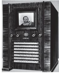
Fig. 13. Lorenz television receiver from 1936 with the television tube invented by Ardenne
