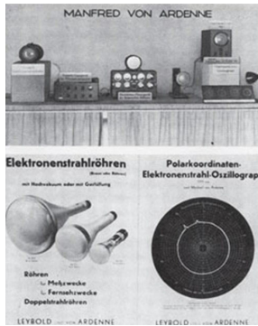
Fig. 16. Berlin Television Exhibition 1936. Above is the stand of the Lichterfeld Laboratory: on the right is a model of a polar-coordinated oscilloscope for radar; on the left are indicators on the Ardenne tubes. Below are two designs of the Leibold and von Ardenne association.
