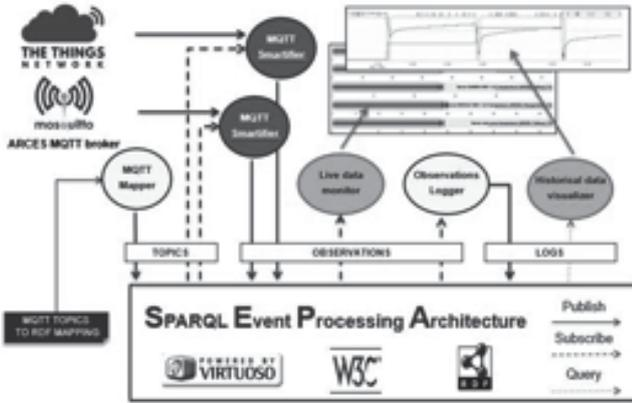
Fig. 3. Sensor data are encoded into RDF triples by MQTT Smartifiers (one for each MQTT broker). The rule for the mapping of MQTT messages into RDF triples are specified into SEPA.
