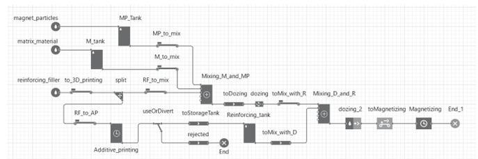
Fig. 3. Simulation model of the experimental Smart Factory
