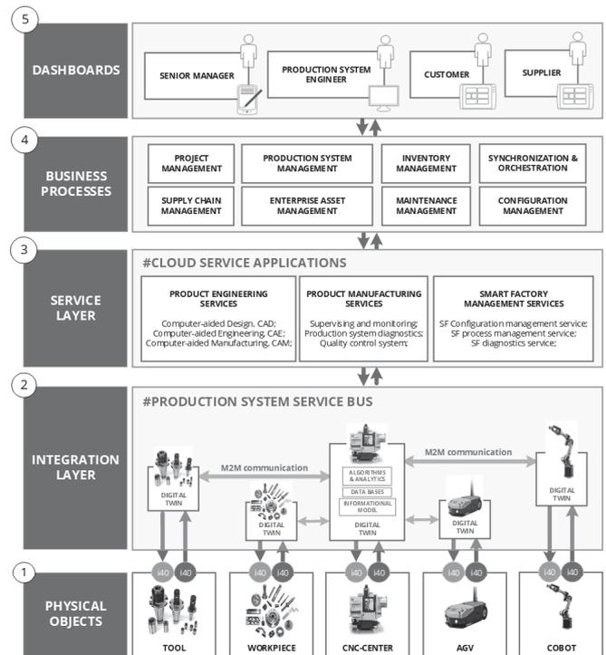
Fig. 1. System architecture of the experimental Smart Factory
