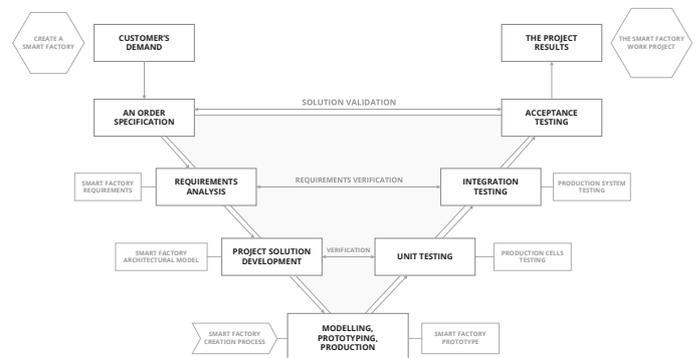
Fig. 2. V-design model of the experimental Smart Factory
