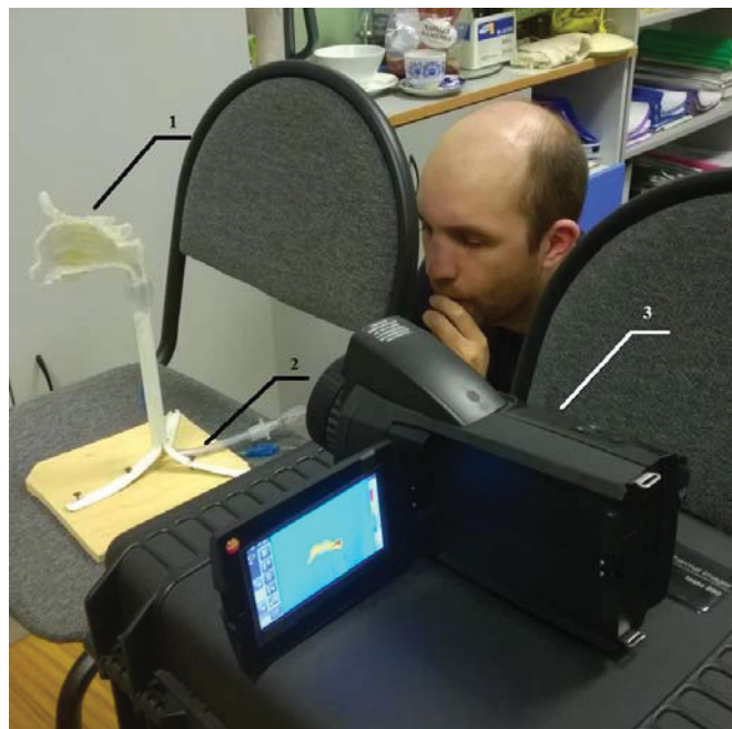
Fig. 3. An experimental stand for measuring temperature field in a solid-state model of the nose, where 1 is a solid-state model of the nose, 2 is an outlet tube for breathing simulation, 3 is a Testo 890 thermal imager
