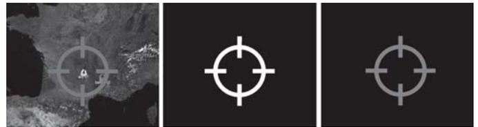
Fig. 2. From left to right; the original screenshot of the interface, the calculated mask, and the final image with the mask applied. Note that the template is preserved without modifications by the mask, while the rest of the interface is hidden
