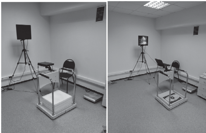
Fig.1. Photography of the stabilography apparatus with (left) and without foam pad (right).
