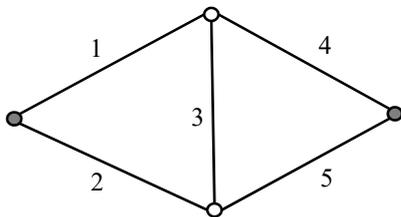
Fig. 2. The example of a network (bridge system)
