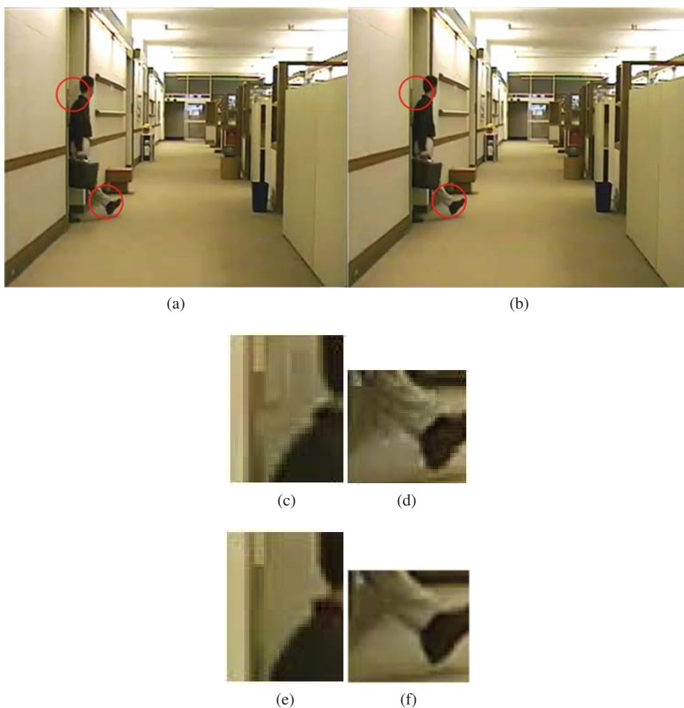
Fig. 5: For video hall , (a) is the 23rd frame of the output video from H.264/AVC compression system with enabled constant bitrate control, (b) is the 23rd frame of the output video from joint VBM3D pre-filtering and H.264/AVC compression system with enabled constant bitrate control, (c) and (d) are highlights from (a),(e) and (f) are highlights from (b).
