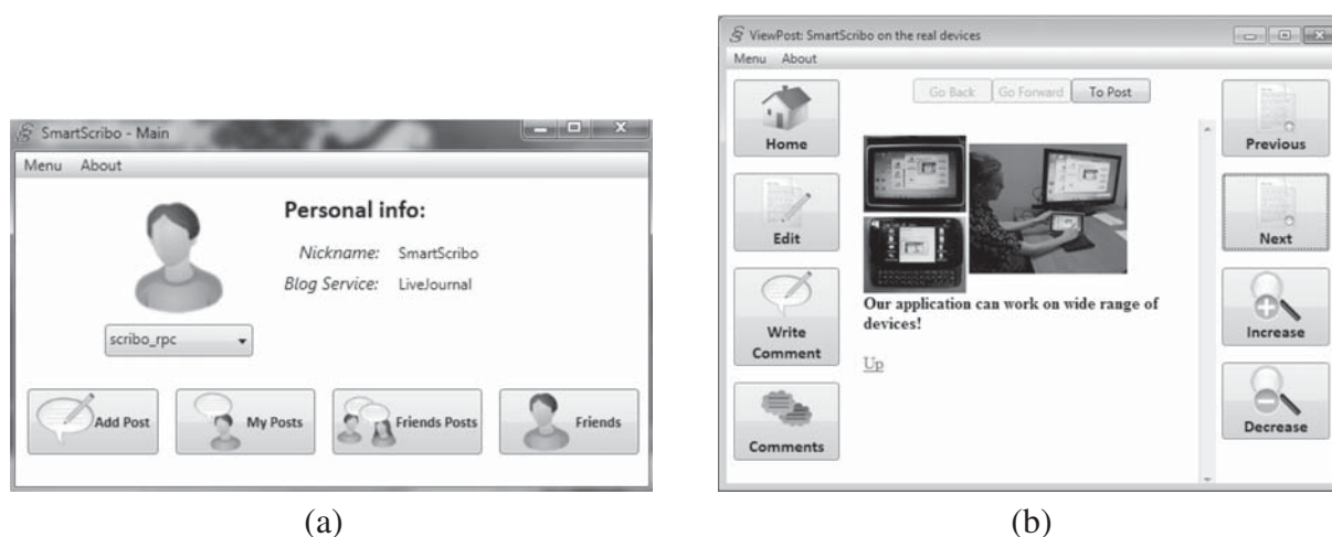
Fig. 1. SmartScribo client GUI for Windows 7. (a) The main client window on a device with landscape screen orientation. (b) The post view window on a device with square-like screen.
