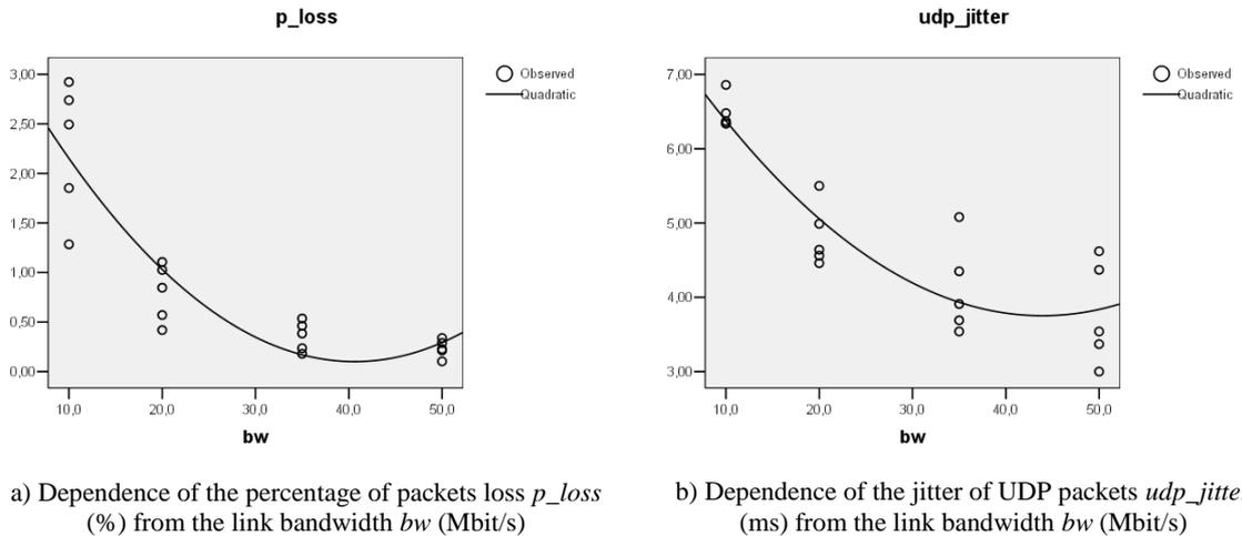
Fig. 7. Dependencies of packets loss percentage and UDP packets jitter from the link bandwidth
