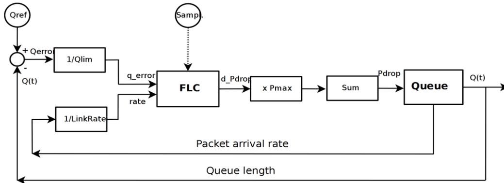
Fig. 1. The structure of the queue management module
