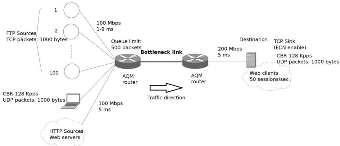
Fig. 4. Network diagram for simulation in NS-2
