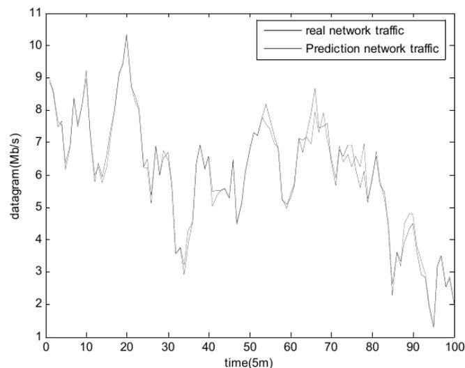
Fig. 2. Five-step prediction of wavelet-neural network
