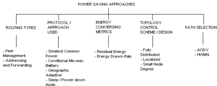
Fig.2. Power save rouging diagram
