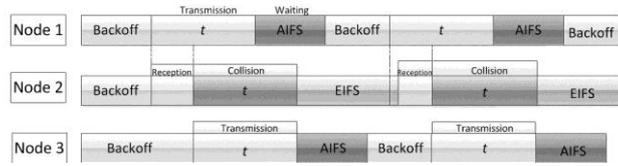
Fig. 7. Vulnerable Node (Asynchronous Case)
