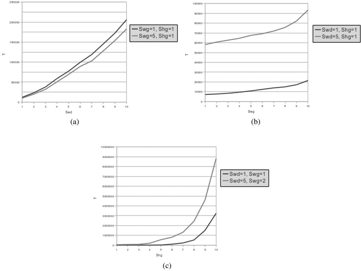
Fig. 3. The measured dependency  $T(s_{wg}, s_{wd}, s_{hg})$ . (a) Variation of  $s_{wd}$  with fixed  $s_{wh}$  and  $s_{hg}$ . (b) Variation of  $s_{wg}$  with fixed  $s_{wd}$  and  $s_{hg}$ . (c) Variation of  $s_{hg}$  with fixed  $s_{wg}$  and  $s_{wd}$ .
