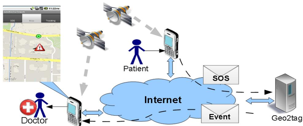
Fig. 2. Client-server architecture of the service
