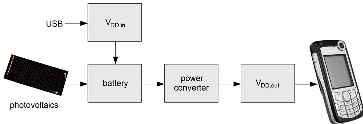
Fig. 3. Components of the Patona 7-in-1 PV charger
