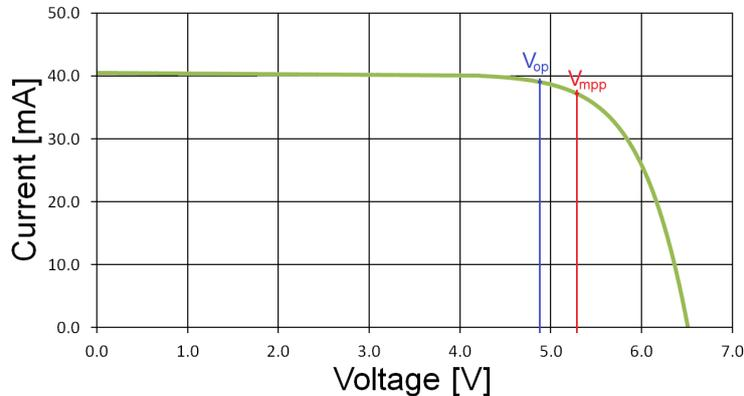
Fig. 4. I-V curve of the Patona 7-in-1 PV charger
