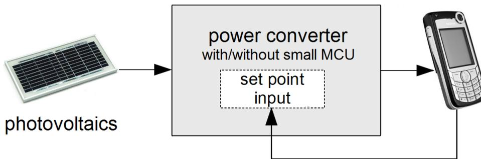
Fig. 9. Proposed connection of photovoltaics with mobile phones
