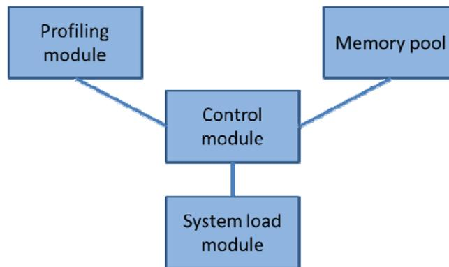
Fig.2. Kernel driver components
