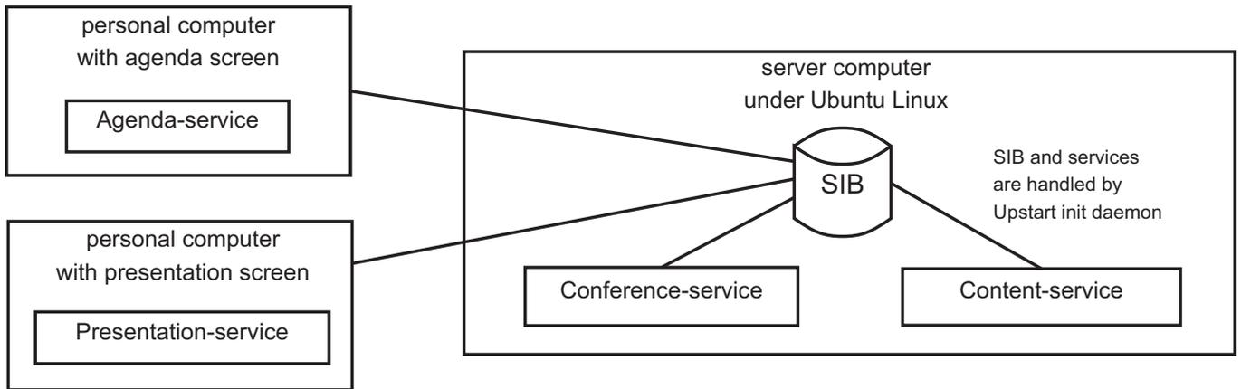
Fig. 1. Scheme of SmartRoom infrastructure on top of Smart-M3
