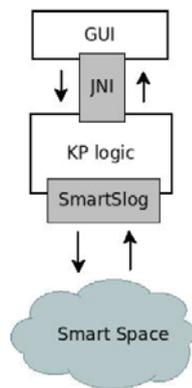
Fig. 2. Structure of Android client KP code: Java-based GUI is connected with C-written client application logic by JNI, SmartSlog ontology library provides domain-oriented data structures and operations for accessing the smart space.
