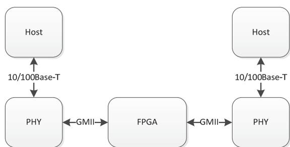
Fig. 2 Specialized Ethernet switch platform
