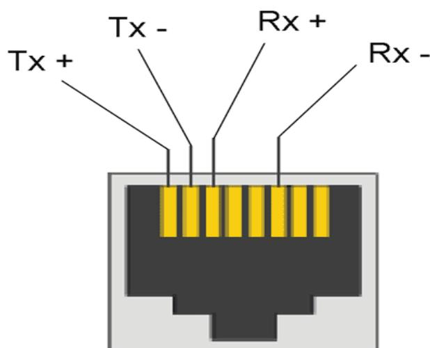
Fig.1 Signals transfer in 10/100Base-T
