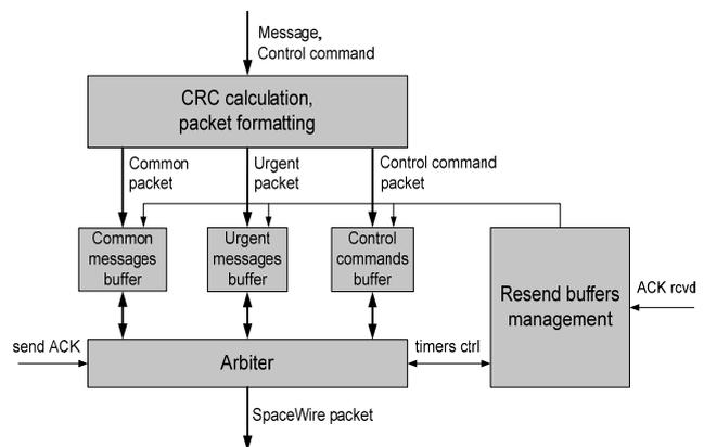
Fig. 7. STP-ISS resend buffers
