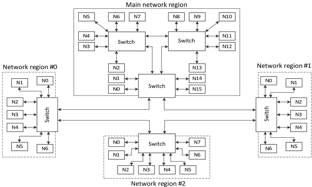
Fig. 2. An example of the onboard network topology with regions
