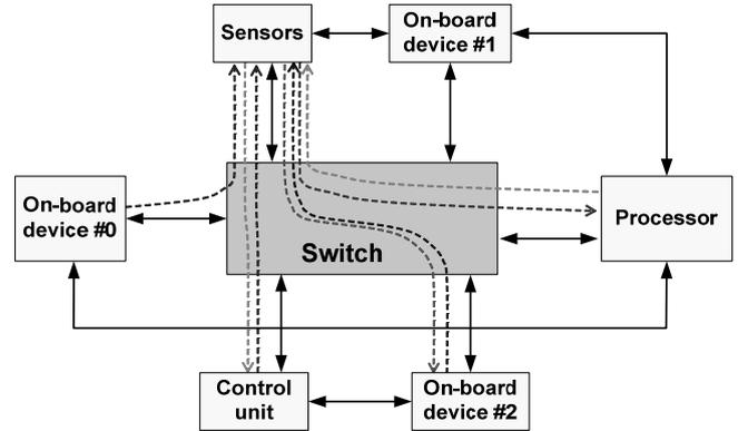
Fig. 1. An example of the onboard network topology
