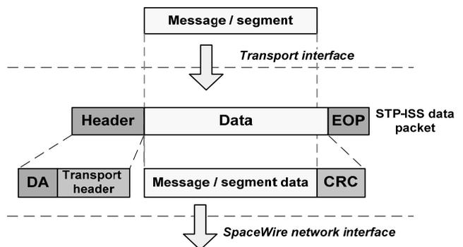
Fig. 5. STP-ISS encapsulation of a message into a SpaceWire packet
