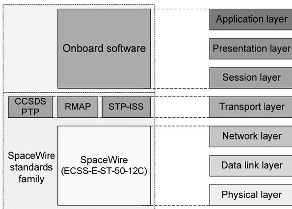
Fig. 3. STP-ISS protocol and OSI model
