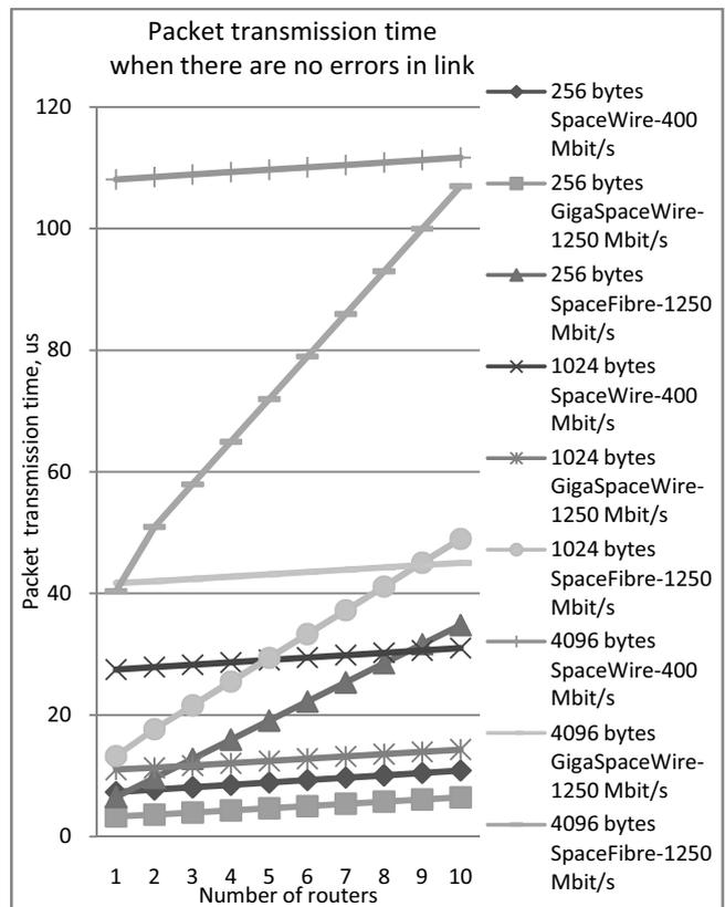
Fig. 8. Dependency between the packet transmission time and the amount of transit routers (without errors during transmission)
