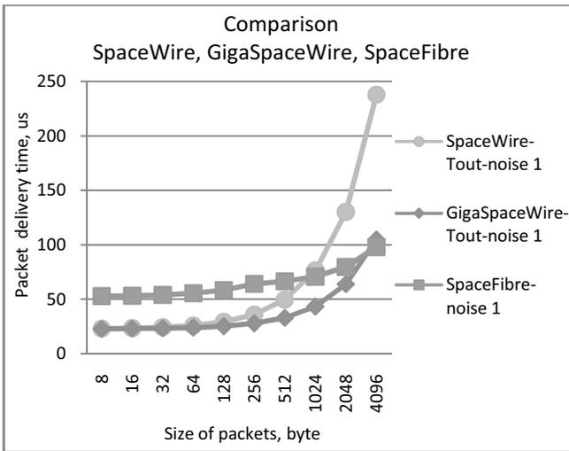
Fig. 6. Dependency between the packet delivery time and the packet size when a transmission error occurs ( $T_{out} = T_f$ )
