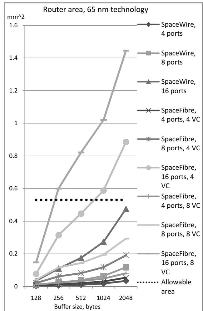
Fig. 11. Hardware cost of base router for different standarts
