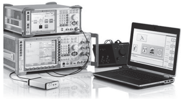
Fig. 2. Conformance testing solution for eCall/ERA-Glonass implemented by Rohde&Schwartz GmbH&Co
