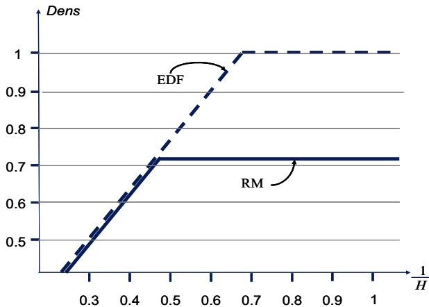
Fig. 2. Hardness/density dependences for EDF and RM scheduling modes
