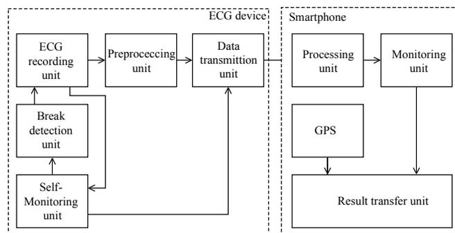
Fig. 2. ECG device scheme
