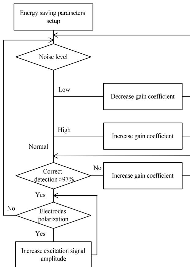
Fig. 9 – Energy saving setup algorithm scheme
