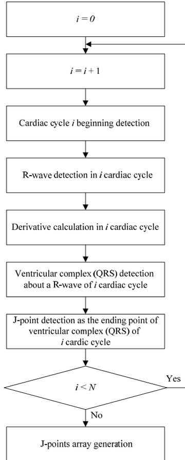
Fig 5. J-point detection algorithm scheme
