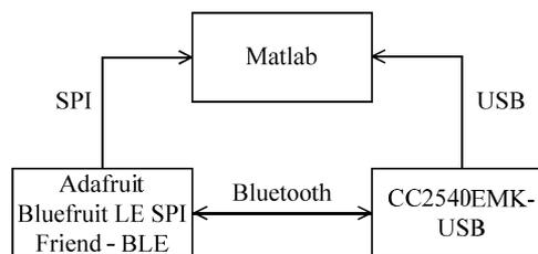
Fig. 10. Wireless protocol test scheme
