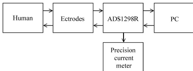
Fig. 8 – Electrode contact break detection experiment scheme
