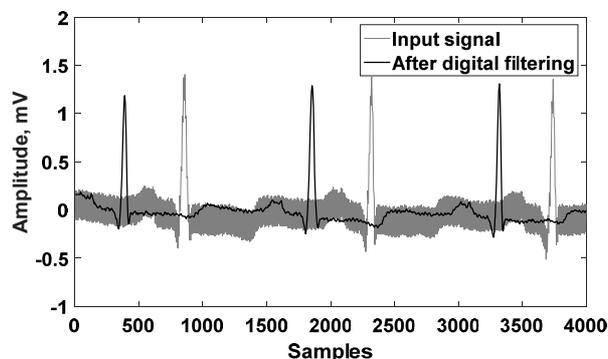
Fig. 7 – ECG in the frequency method of Electrode contact break detection
