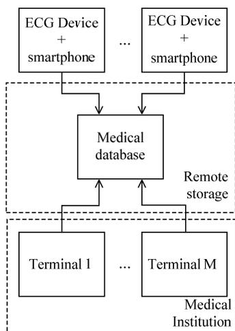
Fig. 1. Heart monitoring system scheme
