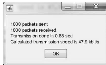
Fig. 11. Wireless protocol bandwidth test results
