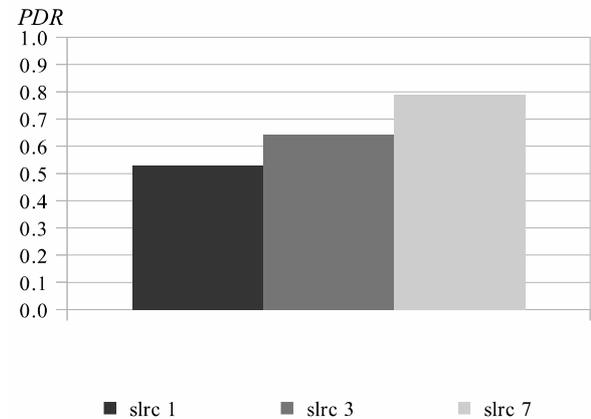
Fig. 6. Measurement results for “fixed-wing drone” scenario. Average packet delivery ratio ( $PDR_{ave}$ ) for each  $slrc$  value
