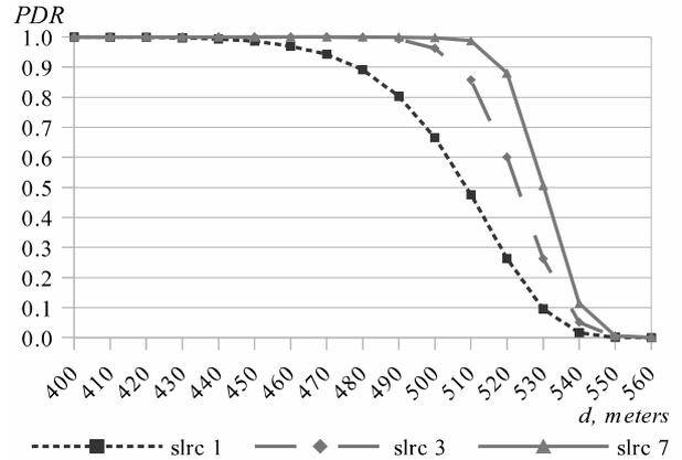
Fig. 5. Measurement results for “quadrocopter” scenario. Average packet delivery ratio ( $PDR_{ave}$ ) for each  $slrc$  value
