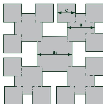
Fig. 11. Fractal antenna of the second iteration
