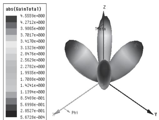
Fig. 13. The radiation pattern on the second radiation frequency
