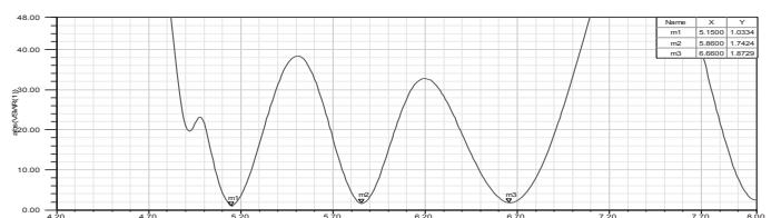
Fig. 17. VSWR of the calculation model of the fractal antenna
