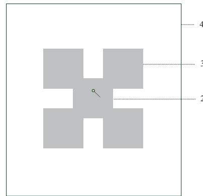
Fig. 1. Fractal microstrip antenna. Top view
