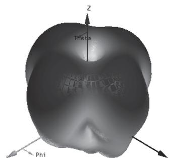
Fig. 12. Radiation pattern on the second radiation frequency (in dB)
