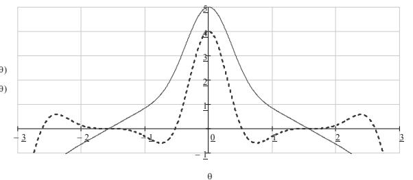
Fig. 10. Normalized radiation pattern of fractal antenna and antenna array 2x2
