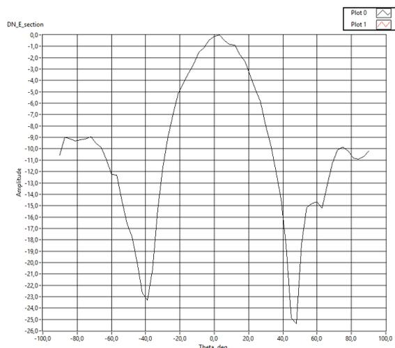
Fig. 19. Radiation pattern of experimental model of the fractal antenna
