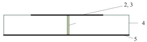
Fig. 2. Fractal microstrip antenna. Side view
