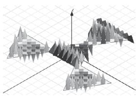
Fig. 5. Distribution of the electromagnetic field in the triangular patch
