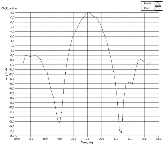
Fig. 19. Radiation pattern of experimental model of the fractal antenna
