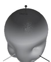
Fig. 7. Radiation pattern of the circular patch
