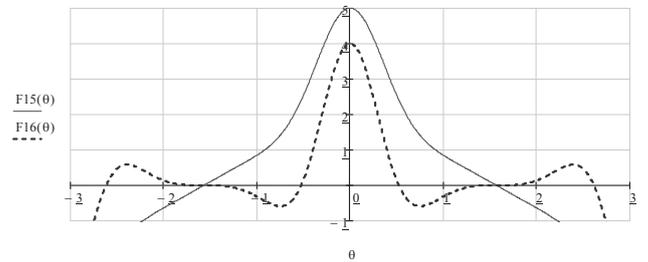
Fig. 10. Normalized radiation pattern of fractal antenna and antenna array 2x2
