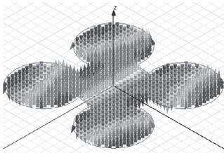
Fig. 4. Distribution of the electromagnetic field in the circular patch
