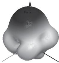
Fig. 6. Radiation pattern of the rectangular patch
