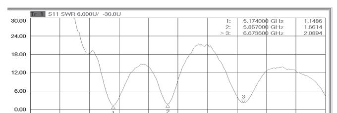
Fig. 18. VSWR of the experimental model of the fractal antenna
