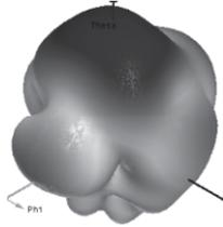
Fig. 8. Radiation pattern of the triangular patch
