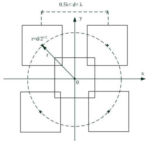
Fig. 9. View of fractal antenna, based on the approach of circular antenna arrays
