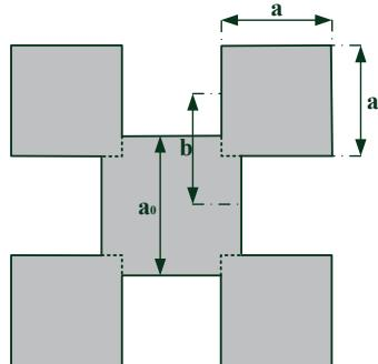
Fig. 15. Fractal antenna with the control geometrical parameters
