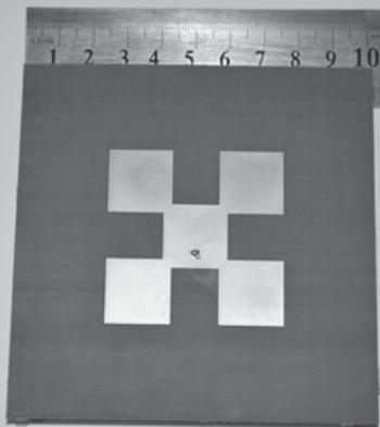
Fig. 16. View of experimental fractal antenna
