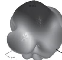
Fig. 8. Radiation pattern of the triangular patch
