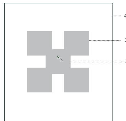
Fig. 1. Fractal microstrip antenna. Top view
