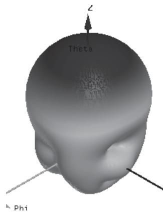
Fig. 14. The radiation pattern on the first radiation frequency of the rectangular based fractal antenna
