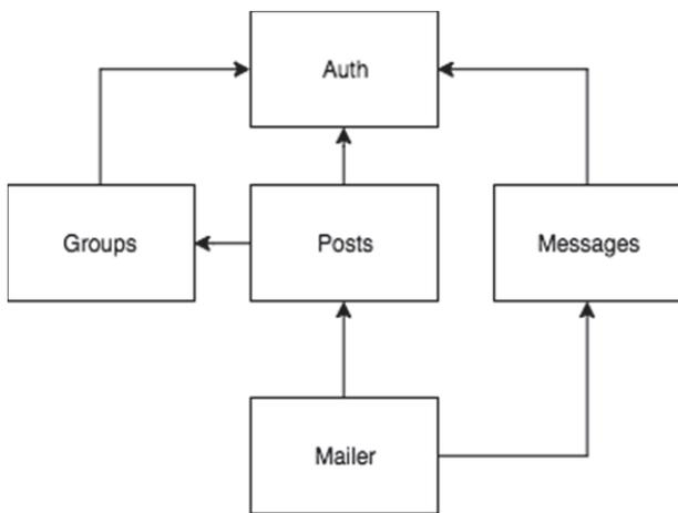
Fig. 4. The block diagram of the micro-service application architecture
