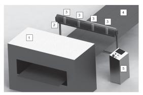
Fig. 2. Arrangement of the complex on the production line, where: 1 - slitting machine, 2 - bearing frame, 3 - cameras, 4 - corrugated board web with cuts, 5 - operator station
