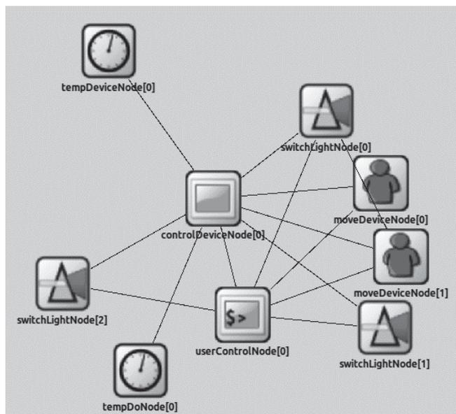
Fig. 3. A simplified model of “Smart home” system in the IDE OMNeT++
