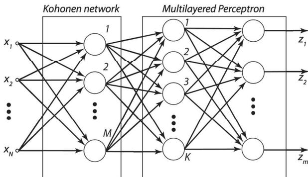
Fig. 2. Structure of Hybrid Neural Network
