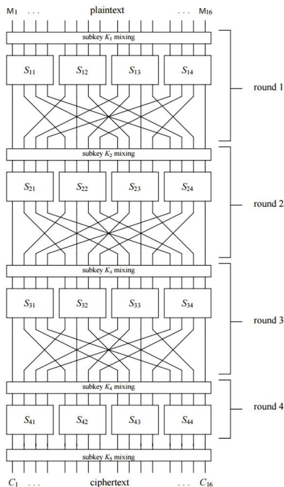
Fig. 1. Substitution-permutation block cipher with block length 16 and four rounds.
