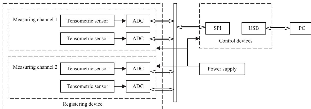
Fig. 1. Block diagram of the tensometric analyzer
