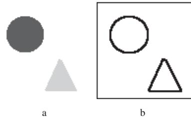
Fig. 1. a – simple objects; b – the same image after Sobel operator
