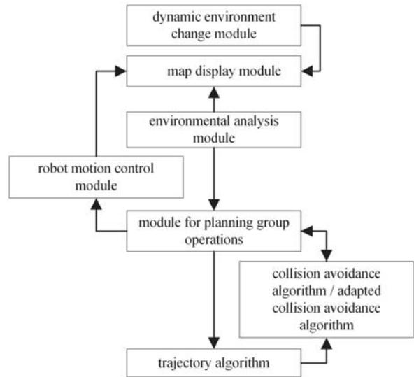
Fig. 3. Interconnection of the module
