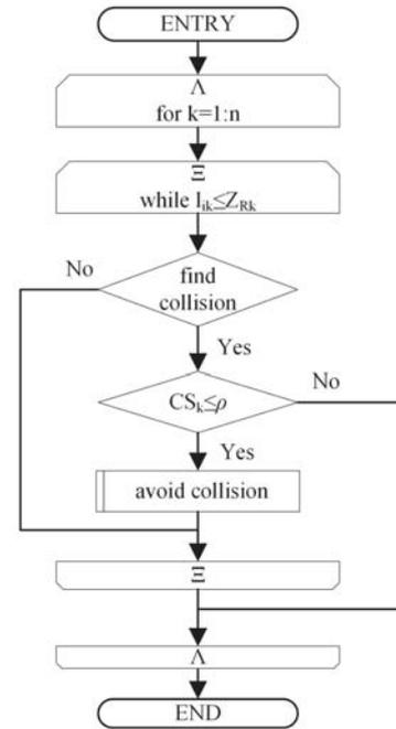
Fig. 1. Adaptive collision avoidance algorithm
