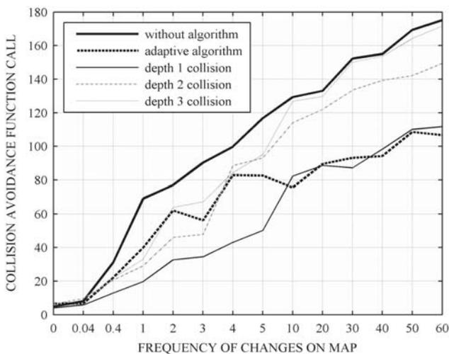
Fig. 6. Collision avoidance function calls
