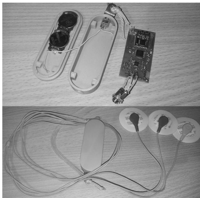
Fig. 2. ECG device prototype
