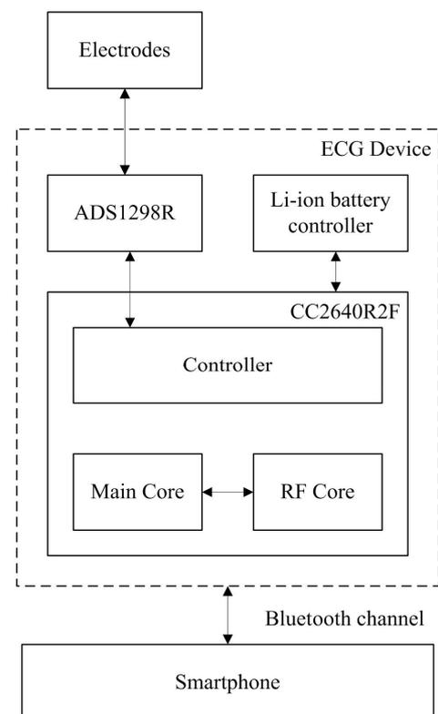
Fig. 1. ECG device structure
