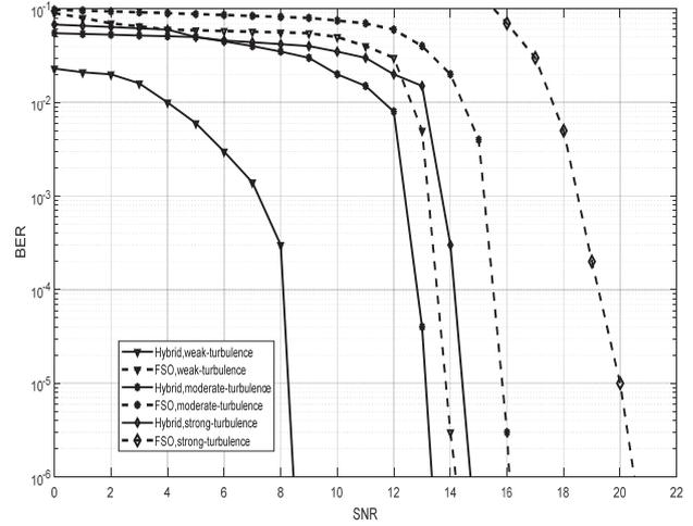
Fig. 4. BER performance comparison of the proposed hybrid FSO/RF system and FSO only system under various turbulence channel conditions
