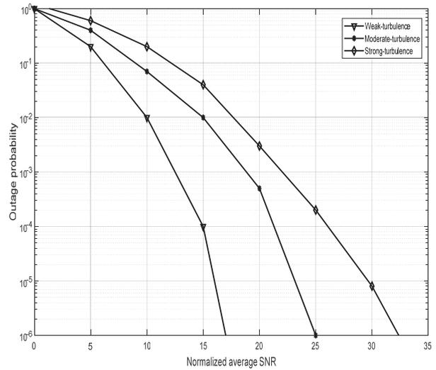
Fig. 5. Outage probability performances of the proposed hybrid FSO/RF under various turbulence channel conditions
