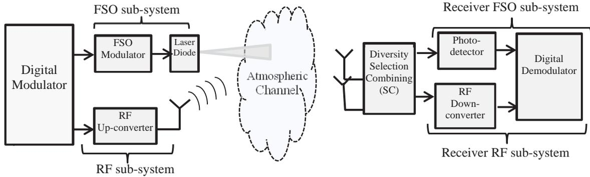
Fig. 1. The proposed hybrid FSO /RF system model block diagram
