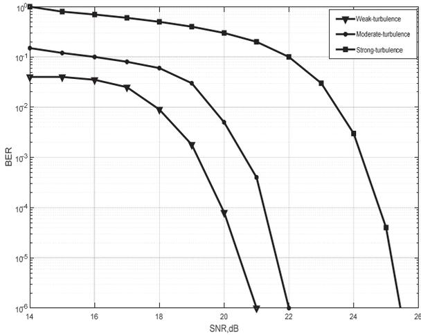
Fig. 2. Average BER performances of the proposed hybrid FSO/RF system under various turbulence channel condition
