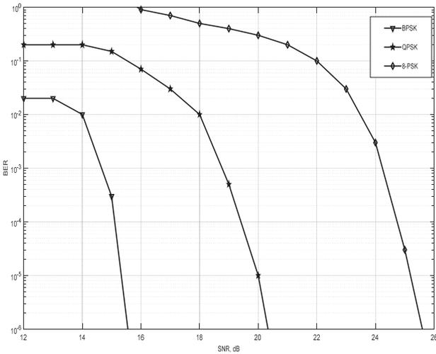
Fig. 3. Average BER of the proposed hybrid FSO/RF system with (BPSK, QPSK, 8PSK) modulation scheme under strong turbulence channel conditions
