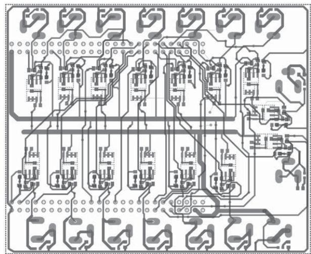
Fig. 4. Layout of Power Distribution Unit
