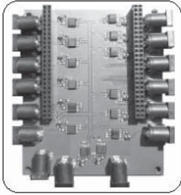
Fig. 6. PCB: Power Distribution Unit
