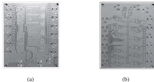
Fig. 5. PCB: Power Distribution Unit (a) Front View (b) Back View
