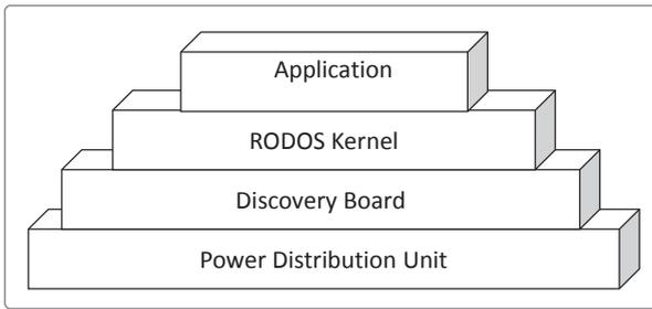
Fig. 1. Conceptual Diagram of the PDU module
