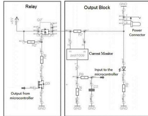
Fig. 3. Electrical Circuit of Each Node in PDU
