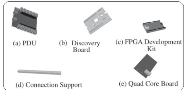
Fig. 9. 3D models of Components of the PDU
