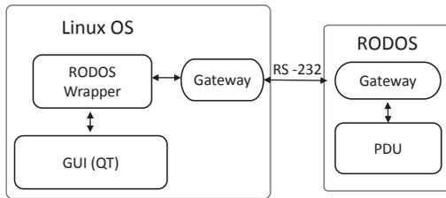
Fig. 18. Communication between PDU and GUI
