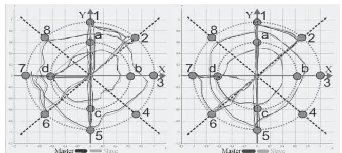
Fig. 8. Trajectory of RJo's handle (Master) and Surikat (Slave) in the absence (left) and presence (right) of force feedback
