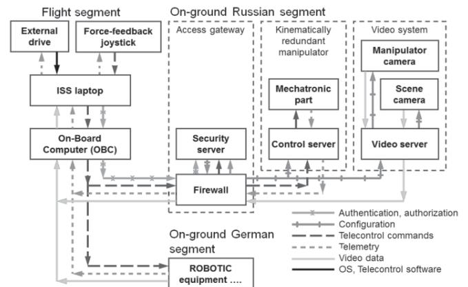
Fig. 6. Functional scheme of space experiment "Kontur-2"
