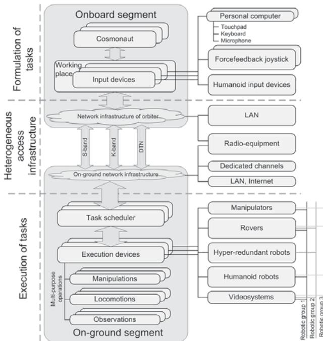
Fig. 12. Data streams in future space experiment "Kontur-3"
