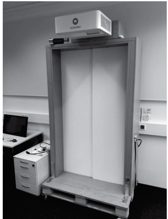
Fig. 4. Prototype of interactive EDS solution on mock-up elevator door
