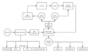
Fig. 3. The process of ML algorithm
