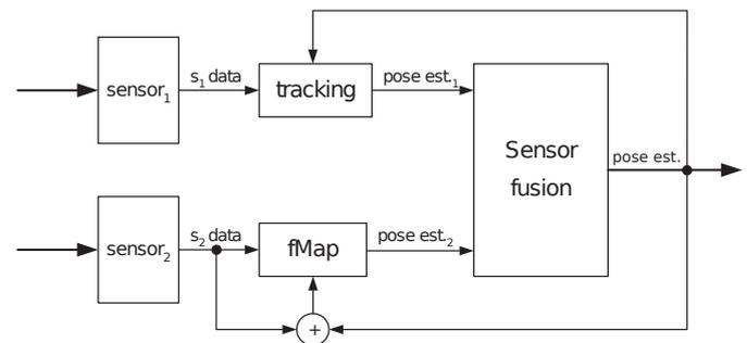
Fig. 1. The high-level scheme of a laser scan based SLAM
