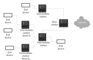
Fig. 1. An example of mesh network nodes connection
