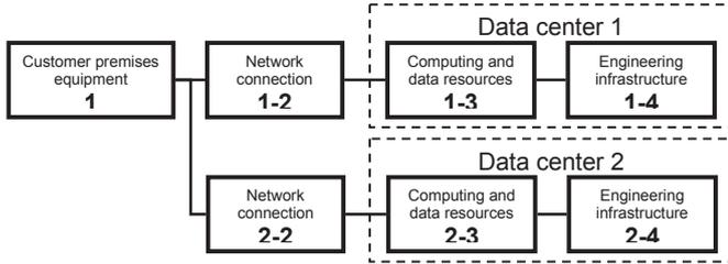
Fig. 3. The block diagram with data center redundancy
