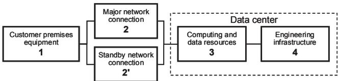
Fig. 2. The block diagram with network connection redundancy
