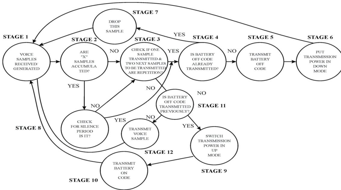
Fig. 4. State Transition Diagram for DITMC at mobile station
