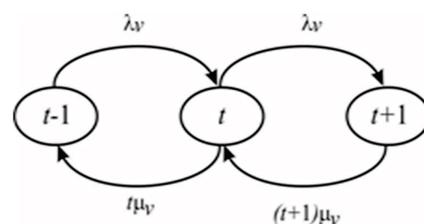
Fig. 1. Markov chain for the voice traffic model with discrete time-slots  $t$ .
