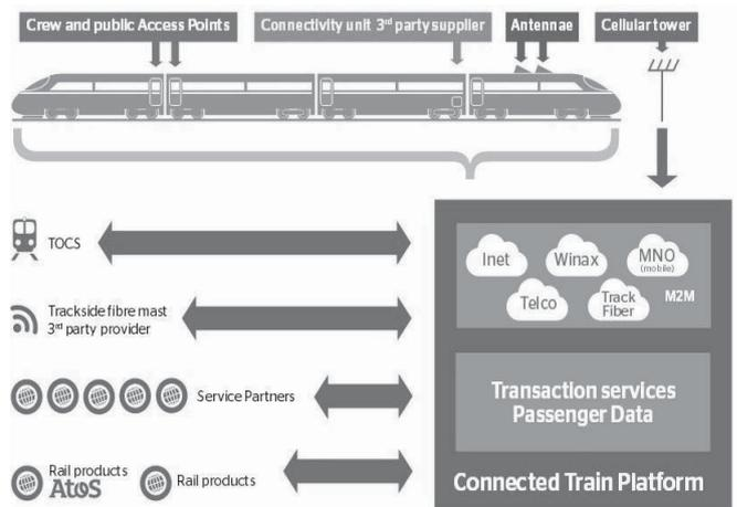
Fig. 6. Connected train platform [13]
