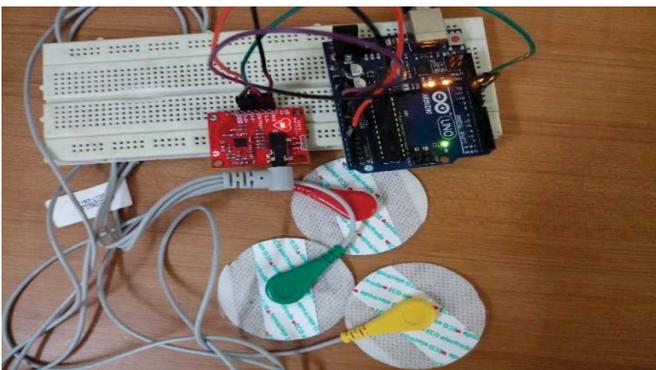
Fig. 3. Connections between ECG Sensor and Arduino
