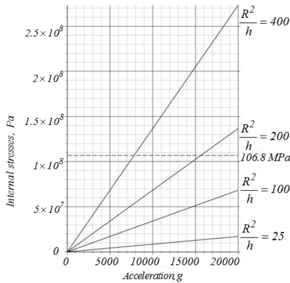
Fig. 8, b. Graph of internal stresses of sensitive elements of lithium niobate YX-128°-cut for the proposed size relationships
