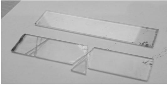
Fig.6. Samples of plates of ST-cut of quartz and lithium niobate of cut YX-128°
