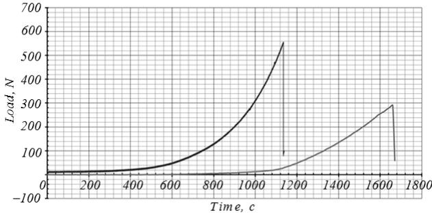
Fig.7. Graphs of the dependence of the load on time for quartz samples of the ST-cut (blue line) and lithium niobate of the YX-128 cut (red line).
