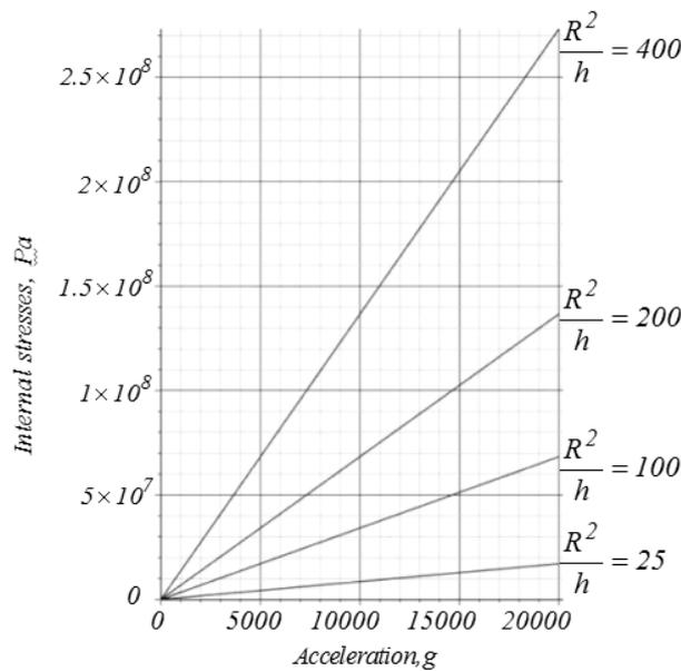
Fig.4, b. Graph of internal stresses of sensitive elements of lithium niobate YX-128°-cut for the proposed size relationships
