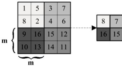
Fig. 2. The max pooling procedure for feature map
