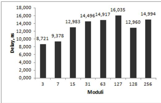
Fig. 8. Delay of convolution operation for different moduli values
