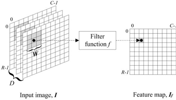
Fig. 1. The procedure for feature maps obtaining
