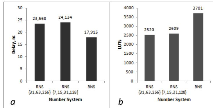
Fig. 9. Simulation results of convolutional layer hardware realization: (a) delay; (b) number of occupied LUTs.
