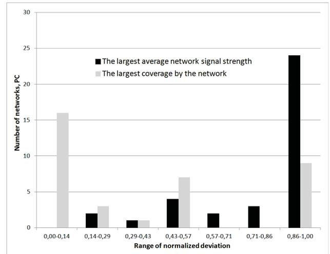
Fig. 7. Error distribution of the method of the largest average signal level of the network and the method of the largest coverage of the network
