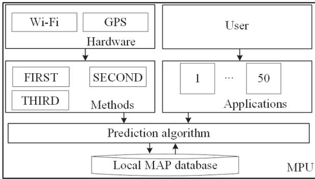
Fig. 4. Scheme of the experiment for analyzing network selection errors
