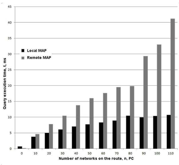
Fig. 9. Dependence of the query execution time on the number of networks for the local and global map location
