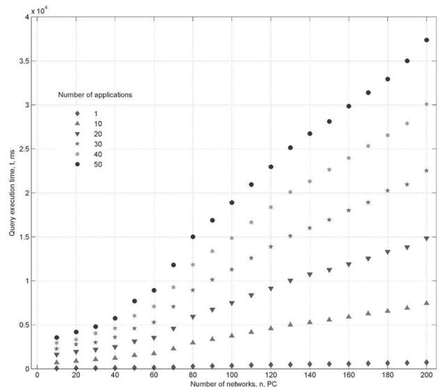
Fig. 3. Dependence of execution time of the prediction algorithm on the number of networks
