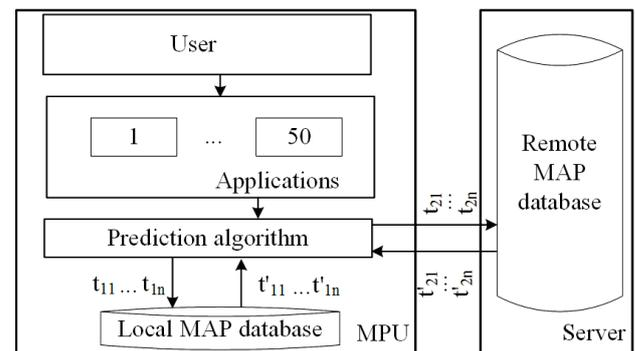
Fig. 8. Scheme of the experiment for the query time analysis to the local and global databases
