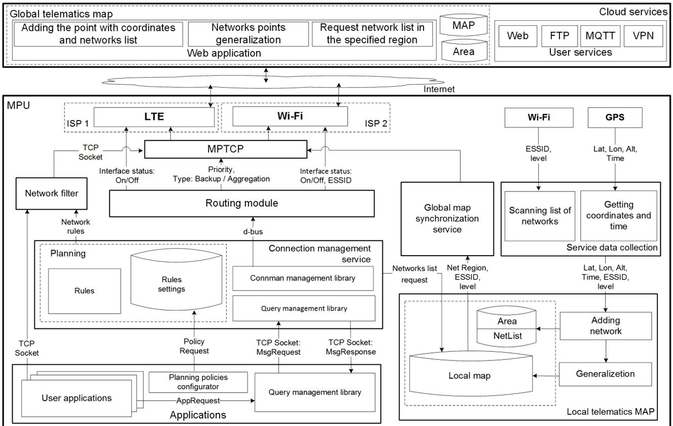
Fig. 1. The architecture of the connection management system
