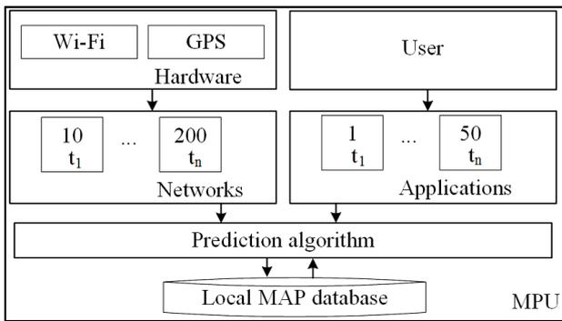
Fig. 2. Scheme of the experiment for analyzing the execution time of the prediction algorithm
